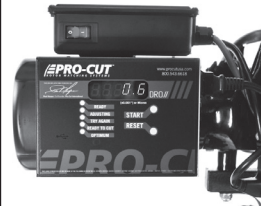
DRO computer compensated for lateral run-out to 0.0006" and ready to cut.
