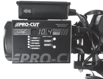
| This value represents hours and tenths of an hour that the motor has to run.
