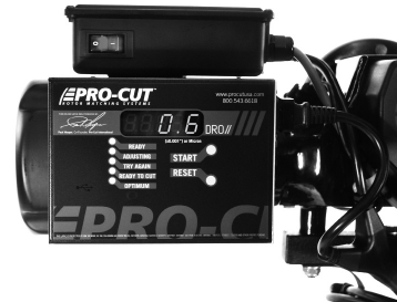
| This display of final compensation equals .0006"
