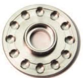
Pro-Cut has updated **50-1403**, the Flange Face. The old unit had two pilot holes where the adapter pin fit; the new unit has 12 holes and a channel for the adapter pin to ride until it beds into one of the holes. The revision allows for easy mating of the lathe between the flange face and the adapter pin, increasing efficiency of setup.
