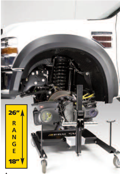
▲ Pro-Cut's PFM 9.2SL with Low-Boy Trolley machining a F-550 SuperDuty truck.
