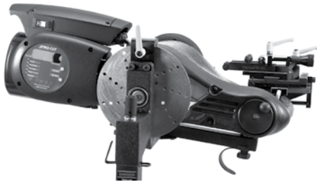
FIG:1 | Lathe in upright position. Note that adjustments to cutting head are simpler in this position.
