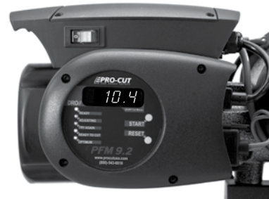
| This value represents hours and tenths of an hour that the motor has to run.
