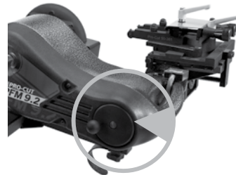
Move the cutting head by turning the knob shown above, clockwise for away from the rotor, counter-clockwise for towards the rotor.
