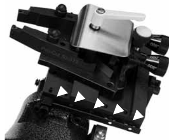
| Detail of the gib adjustment screws
